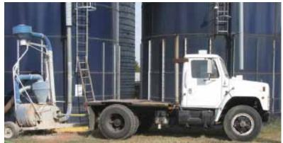
This 200 hp plus truck is attached to a grain-vac. Notice the pto gear box and the live hydraulics (below).
