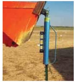
Zweifel's T-post driver hangs from the front edge of loader bucket.
