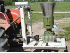
Pto-powered pelletizer has a heavier-duty gearbox that'll stand up to increased pelletmaking torque, says the company.
