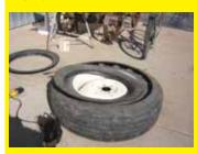
We needed turf tires for our tractor but could not justify them. So we bought some old, bald truck tires that were 1/2 size bigger than the tractor tires. We cut 2 to 2 1/2 in. off the inside of each tire sidewall and slid them onto the tractor tires, then reinflated. Works great and we no longer leave tracks from lugged tires when spraying weeds. (Andy, Delta, Colo.)
