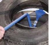
It works because of the patented shape of the tool's head, and the leverage that you get from the handle.
