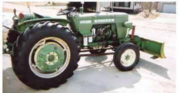
With help from family and friends, Melvin Erskin repowered this old Oliver 1250 tractor with an Isuzu diesel engine.
