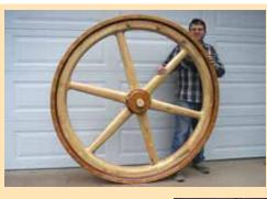
Gary Martin makes models for castings, ranging from miniature parts for antique tractor collectors to man-sized steam engine flywheels.
