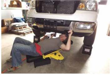
The BatWing is a modern, ergonomic version of a mechanic's creeper. The back is controlled by a gas spring and is made from molded foam cushioning.
