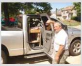
Greg Smith, Pacific, Mo.: Greg came up with a simple solution for tool storage in his crew cab pickup. Although retired, he does a lot of handyman work and likes to have his tools with them. But he didn't want to have a big toolbox in the box. So he made some shelves that simply rest on top of the back seats in the cab. They can be quickly lifted out to make room for grandkids or guns and they protect the seats from damage that would be caused by placing toolboxes directly onto them.
