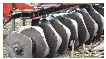
The flat sides on Falk's 5-sided disk blades push crop residue down into the soil surface. Only the points penetrate the soil.
