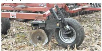
Falk installed a set of the blades on his Case IH 496 28-ft. disk and calls it a Rolling Spader.
