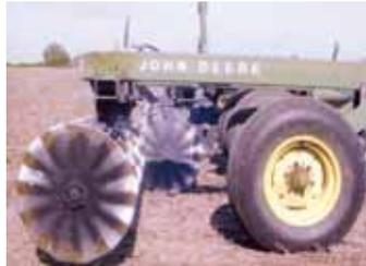
He straightened out the gangs and put straight/wavy coulters on them, both front and back.
