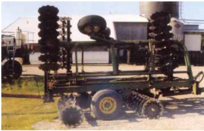
To save the cost of a new vertical tillage tool, Robin Miller modified this Deere 230 disk at a cost of about \$6,000.
