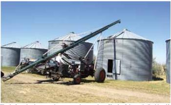
Tired of moving heavy grain augers at harvest time, Charles Johnson built this self-propelled auger. The engine is off a Gleaner combine.
