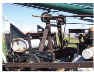
Auger is driven by double groove pulleys from the combine, and its separator clutch stops and starts the auger.
