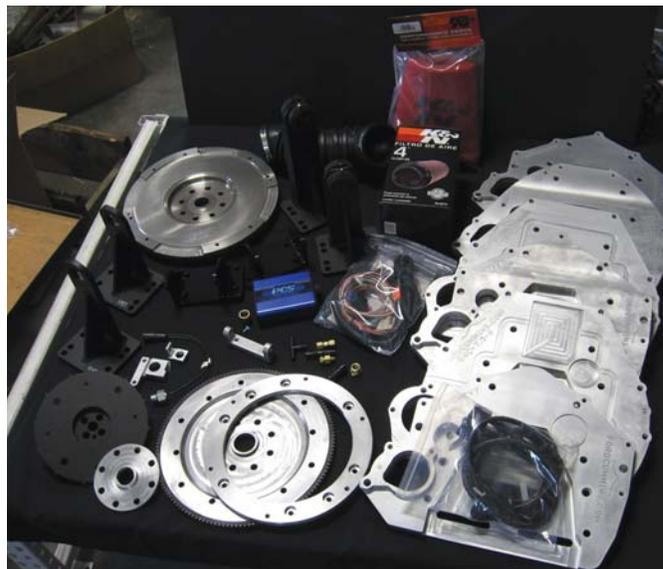
DCS conversion kit is used to convert a Ford engine-powered truck to a Cummins diesel.
