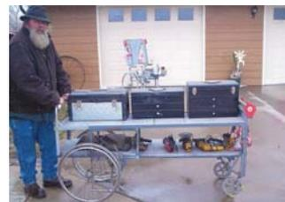
Ken Grazier attached a 6-ft. long bed frame to a set of wheelchair wheels to make this portable work bench.
