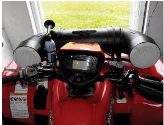
ATV-mounted speaker system uses a section of 6-in. dia. sewer pipe. Amplifier fits inside pipe's straight section, and speakers fit into the ends.
