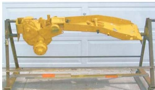
**He uses this stand to work on garden tractors. It has adjustable mounting brackets at either end.**
