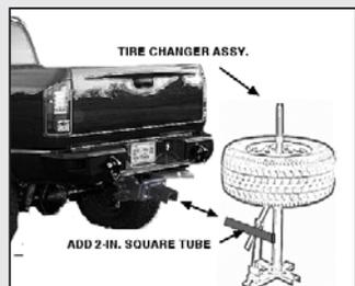
with bead breaker, mount/dismount bars, etc. I take it with me on road trips where I almost always blow a tire or two. I welded a 2-in. sq. tube on the tire changer assembly that fits into my pickup’s receiver hitch. I also welded an extra receiver tube on the tongue of my trailer, which allows me to change tires on the road without having to drop the trailer. It works great and has saved me a lot of money over the years.”
