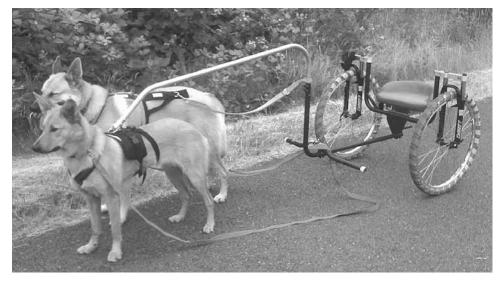
Dog cart has a single shaft that goes over dog's back and pulls upward on harness.
