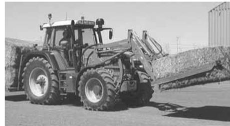
Depending on the model and the tractor/loader combination, an operator can pick up one to six bales at a time.
