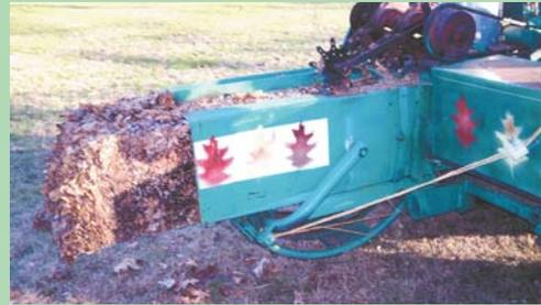
Commercial-sized baler is sized to be pulled behind a compact tractor and produces bales that measure 18 in. wide by 14 in. high.
