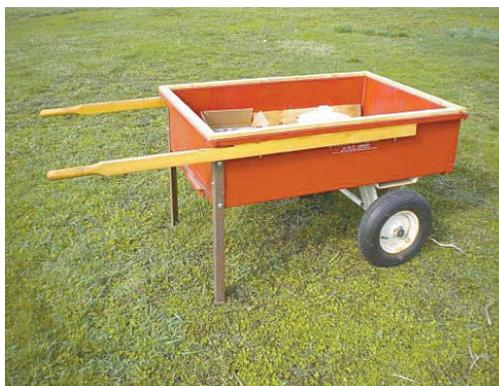
Joseph Parducci converted an old 10 cu. ft. tow-behind cart into this high capacity “wheelbarrow-style” cart.
