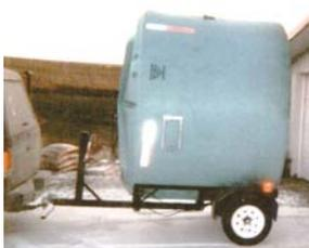
Made from a 1,550-gal. poly tank, Floyd Martin's ice fishing house bolts permanently onto a 2-wheeled trailer for easy transport and setup.
