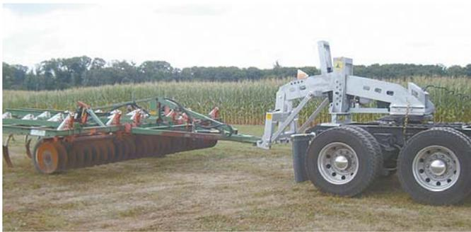
Fifth wheel boom turns a semi tractor into a wrecker/equipment mover, allowing you to quickly move farm equipment from one field to another.
