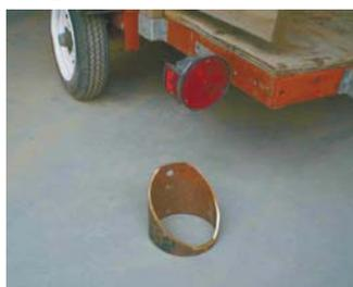
Protector is built from a short length of 6-in. dia. well casing, cross-cut at an angle.
