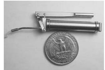
He made a grease gun that's amazingly small - about the size of a quarter to service the tiny Deere D.
