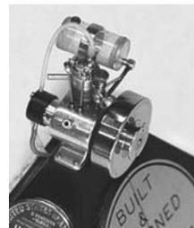
This single cylinder spark plug engine is thought to be the smallest running spark plug-fired gas engine in the world.
