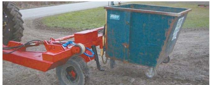
Add-on wheeled dump box works great for hauling split wood. It has a hook on top and its own hydraulic cylinder, allowing Cook to lift box for transport and then dump the wood.
