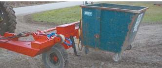
Add-on wheeled dump box works great for hauling split wood. It has a hook on top and its own hydraulic cylinder, allowing Cook to lift box for transport and then dump
