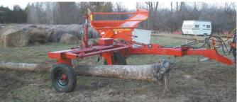
Doug Cook stripped an old mower-conditioner down to the frame, turning it into this low-cost log hauler. It can handle 18-in. dia. logs up to 20 ft. long.
