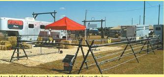
Any kind of fencing can be attached to guides on the legs
