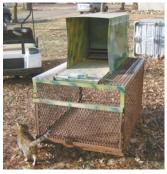
Trap uses a holding cage with a sheet metal box and trigger plate on top. Trigger resets itself after an animal is trapped.
