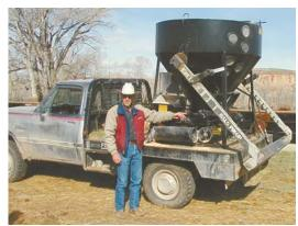
Mix 'N Feed loads, mixes and delivers up to 42 bu. of whole grain and concentrate pellets in a single trip. It can be mounted on a truck or trailer.
