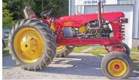
Ed Pacha repowered his Massey Harris 44 tractor with a fuel-injected V-6 engine out of a 1987 Chevy Caprice.
