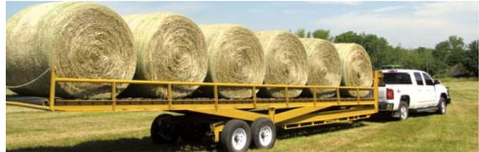
Hayroll trailer is designed so bales can be loaded side-by-side from either side, or end-to-end.
