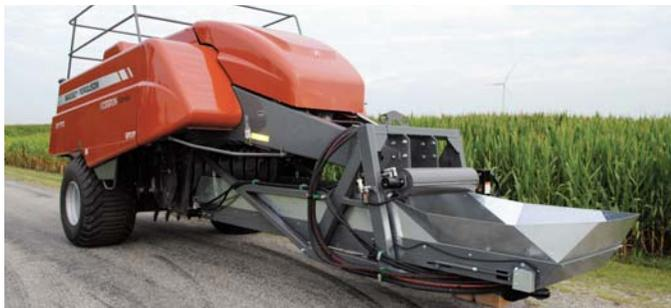
Bolt-on unit allows combine to pull baler, harvesting grain and crop residue at same time. Enclosed conveyor delivers material to baler.
