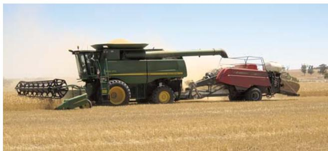
A hydraulic motor, powered by an independent hydraulic pump on combine, drives baler.
