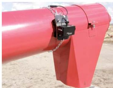
Magnetic camera system helps operator on ground line up auger with opening on top of grain bin.
