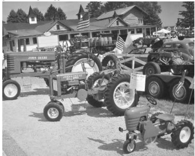
Mini 1935 Deere B is powered by an 8 hp Tecumseh engine (center). Old Murray pedal tractor was converted into a motorized unit powered by a 2 hp Tecumseh engine (right). Note full-size Deere B in background.
