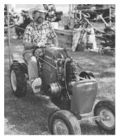
Loren Etter built this "one-lunger" garden tractor by stretching out a Wheelhorse garden tractor and mounting a Cushman engine on it.
