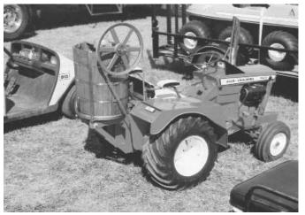
Doug Snider mounted a 5-gal. ice cream maker on back of his Allis Chalmers B10 garden tractor. It's belt-driven off tractor's mower deck.
