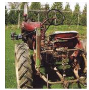
Cable runs from winch back to a clevis mounted on top of a vertical metal bar that's part of tractor's lift system.
