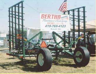
The front and rear half of the Bertha harrow can be hydraulically raised or lowered to prevent gouging and to allow trash to flow through.
