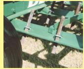
Harrow is equipped with 5 steel bars that support a series of clamp-on, 1-in. heavy steel drag teeth.
