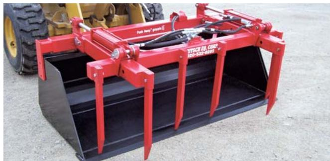
**Push Away Grapple digs into compacted feed and then pushes skidsteer back to keep its wheels from tearing up the ground.**
