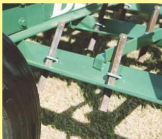
**Harrow is equipped with 5 steel bars that support a series of clamp-on, 1-in. heavy steel drag teeth.**
