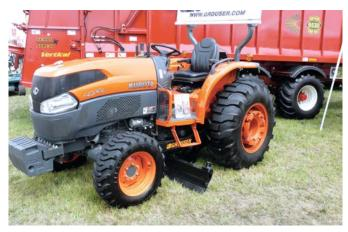
Unlike front or rear-mount blades, the Grouser Belly Blade doesn't hop or leave ripples Five hydraulic cylinders raise, lower, angle, tilt, change pitch and side-shift the blade. behind. And there's no need to look back.
