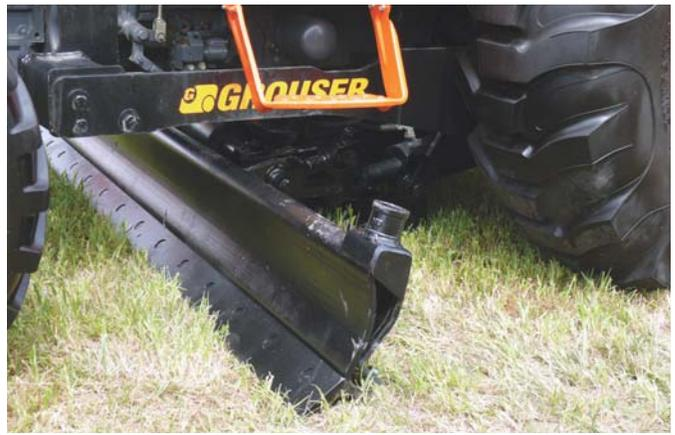
Five hydraulic cylinders raise, lower, angle, tilt, change pitch and side-shift the blade.
