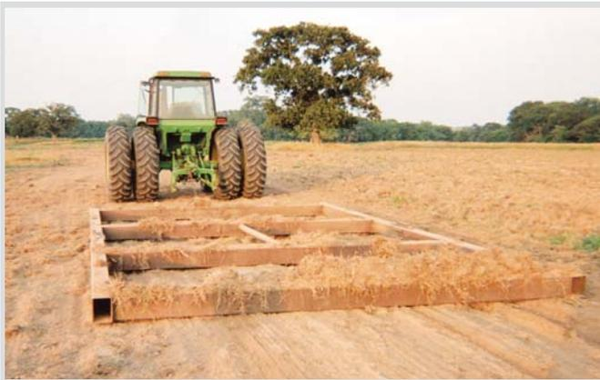
Don Golden needed to smooth out excavation ruts after building a lake on his property, so he built this 13 by 26-ft. drag out of rectangular steel tubing.
