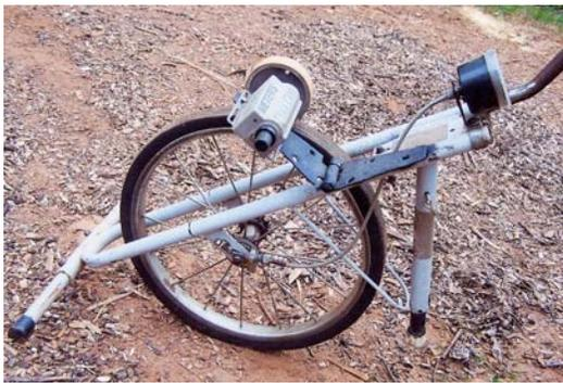
Glenn Fisher made his own measuring wheel by converting an old exercise bike equipped with an 18-in. dia. rubber wheel.
