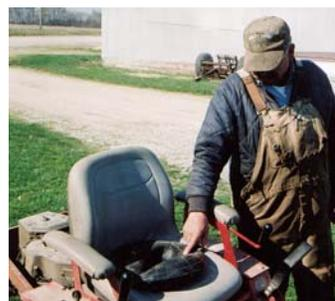
Slightly inflated rubber inner tube sets on mower's bucket-type seat, helping to smooth out bumps while mowing.
