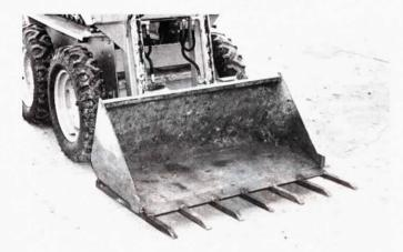
Short chains with built-in tighteners hold clamp-on teeth in place.
