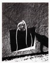
A 1/10 hp. motor spins three nylon "whips" that hit intruding predator in the face.
