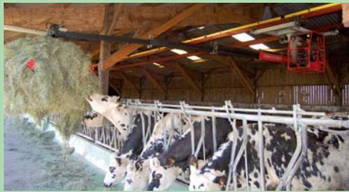
Crane's arm extends up to 30 ft. to grab more than 800 lbs. of hay at a time and place it in front of cows in tie stalls.
