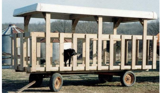
Feeder is built on top of a Case wagon running gear and uses an old pop-up camper top for a roof.
