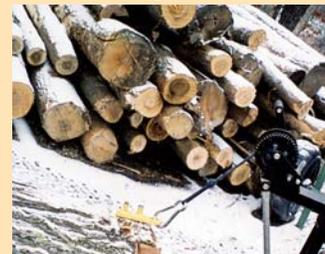
Hand-operated, 2,000-lb. boat winch is used to lift one end of log off ground.
