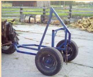
Miller built the arch out of 2-in. sq. tubing, 2-in. flat iron and wheels from an old baler.
