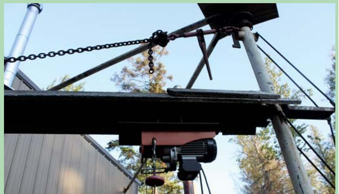
Tower-style log loader consists of a pivoting center post with a 10-ft. boom and a traveling hoist. Struble uses a hand-held remote control to activate hoist to drop "log handle" to log.
