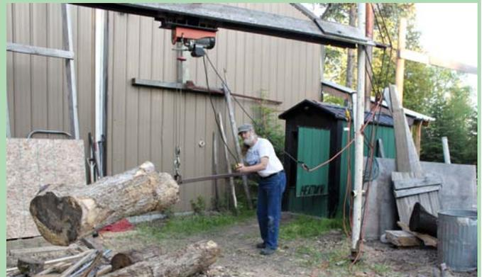
"The problem with big outdoor wood-fired boilers is that it's really hard to slide big chunks of wood in on top of each other. With my home-built log loader, I can do it without even getting smoke in my face," says Jim Struble.
