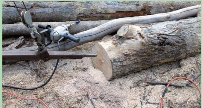
Struble cuts 8-ft. logs in two and drills a 4-in. deep, 1-in. dia. hole in one end of each log.
