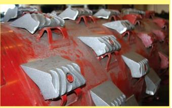
High performance thresh bars are designed for AFX/specialty rotors in Case IH combines. "They work especially well in hard threshing crops," says inventor Ron Kile.
