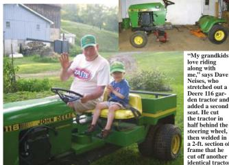
along with me," says Dave Neises, who stretched out a Deere 116 garden tractor and added a second half behind the steering wheel, then welded in 2-ft. section of cut off another identical tractor.
