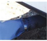
Rigid plastic adapter clamps onto vehicle's exhaust pipe.
