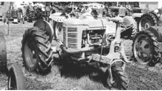
Iky Wipf used components from 4 different tractors to build this "slow speed" tractor. The 4-cyl. industrial engine – bolted crosswise on a Deere frame – is off an Interna-
