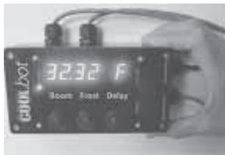
**Coolbot micro-controller checks for frost or freeze-up and adjusts the A/C fan and compressor as needed.**
