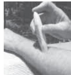
**Electronic Itch Soother uses a heating element to reduce itching sensation.**
