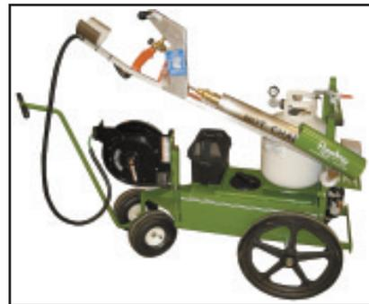
Green Steam machine kills weeds with 660-degree steam. Wheeled cart holds the steam thrower gun, 7-gal. water tank, 20-lb. propane bottle, and battery.
