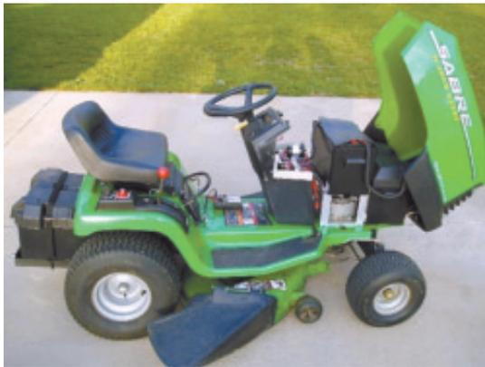
Gary Little converted his 1997 Deere Sabre riding mower to electric power, replacing the 16 hp engine with an Etek DC motor from Briggs & Stratton.
