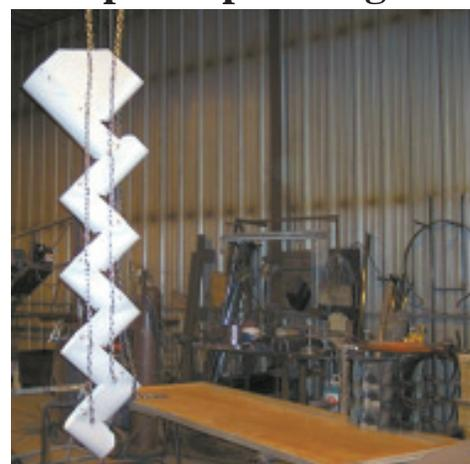
Lorrich seed ladder is made from rubber belting that lasts longer than steel bean "ladders", says the company.
