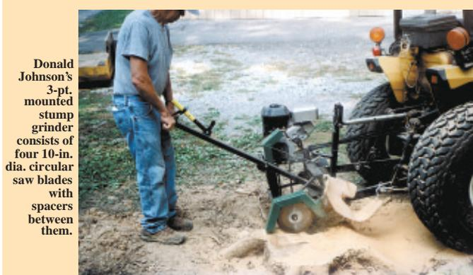
Donald Johnson's 3-pt. mounted stump grinder consists of four 10-in. dia. circular saw blades with spacers between them.
