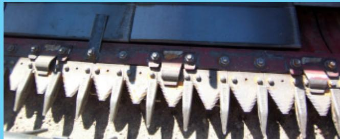
After kit is installed, beans no longer catch on ridge behind cutterbar.
